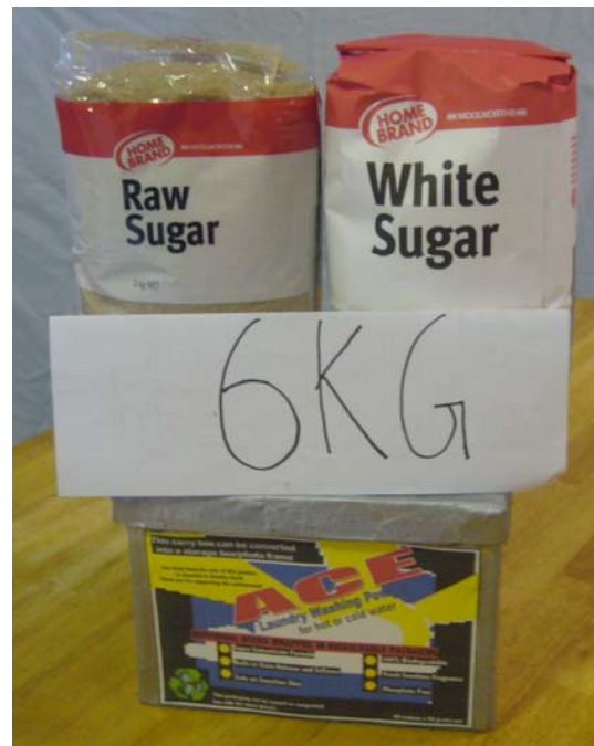
Strength test-showing the prototype easily supporting 6 kilograms. The sugarcane material is currently being used as disposable food containers which proves it can withstand heat.
